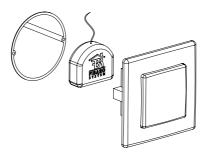
Fig.2 Installation of Fibaro Relay Switch in wall switch box.
