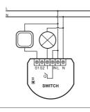
Double switch - mains electricity power connection
