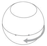
2. Remove the battery blocker.
